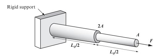
Show that the **total** extension  $\Delta x$  of the bar under the action of an applied force F, as shown in the diagram, can be given by (i)
